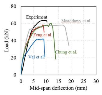
Fig. 4—Bond strength reduction model influence on analytical response of BT1-2-4 beam. (Note: 1 kN = 225 lbf; 1 mm = 0.04 in.)
