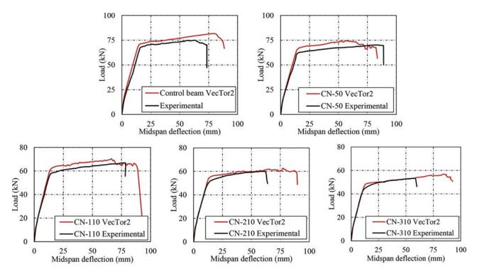
Fig. 5—Experimental versus analytical load-deflection responses for El Maaddawy et al.<sup>30</sup> specimens. (Note: 1 kN = 225 lbf; 1 mm = 0.04 in.)
