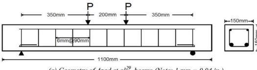
(a) Geometry of Azad et al.<sup>29</sup> beams (Note: 1 mm = 0.04 in.)
