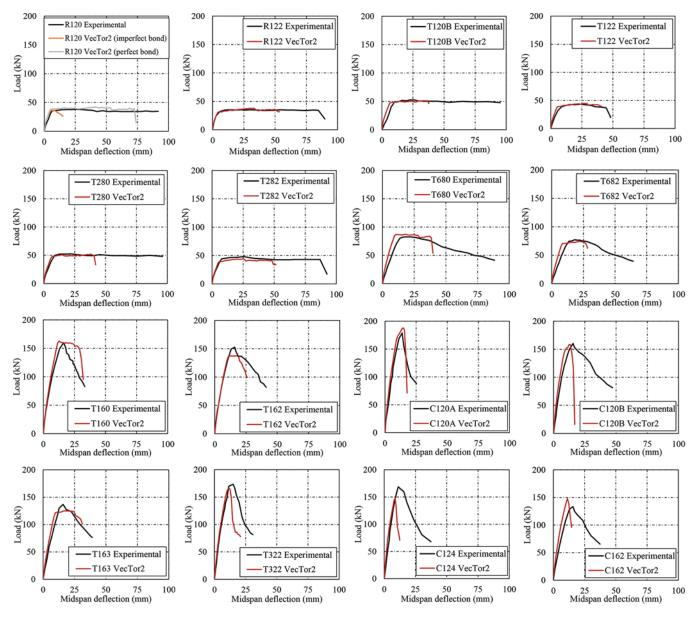
Fig. 7—Experimental versus analytical responses for Du et al.<sup>31</sup> specimens. (Note: 1 kN = 225 lbf; 1 mm = 0.04 in.)
