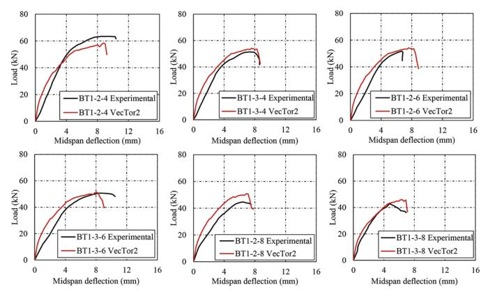
Fig. 3—Experimental versus analytical load-deflection responses for Azad et al.<sup>29</sup> specimens. (Note: 1 kN = 225 lbf; 1 mm = 0.04 in.)
