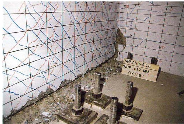
FIGURE 8. DP1-R at Failure
