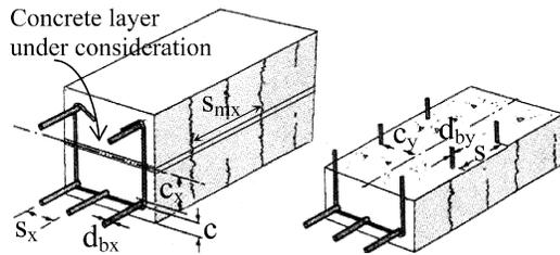
Fig. 12—Parameters influencing crack spacing (adapted from Collins and Mitchell [1991]).
