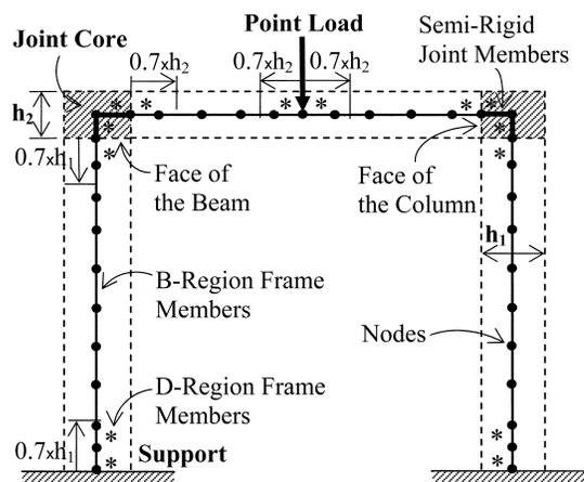
Fig. 11—Frame model with shear-force-reduced D-region members.
