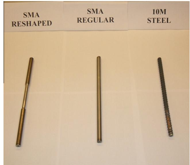
Fig. 3. SMA and conventional reinforcement samples.
