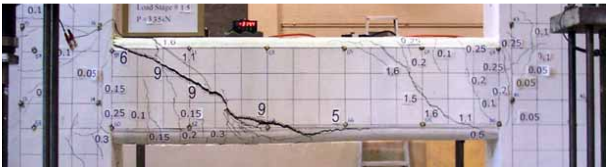
Figure 6.17 Beam Crack Pattern at +40 mm of Top Storey Deflection
