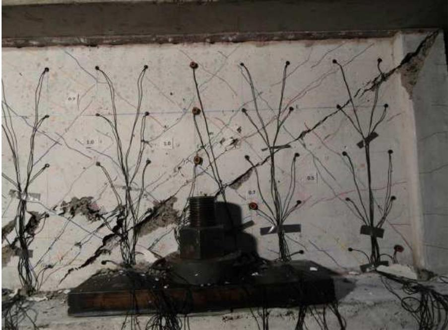
Figure 5.10 – ASR A1 shear wall at failure (Habibi et al., 2015)
