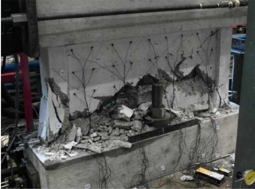
Figure 5.9 – Regular A shear wall at failure (Habibi et al., 2015)
