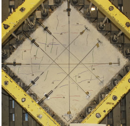
Double Cycle 5, Stage 20: v_{xy} = -3.70 MPa, \gamma_{xy} = -1.22 \times 10^{-3} ; w_{cr,max} = 0.60 mm, w_m = 0.17 mm, s_m = 149 mm.
