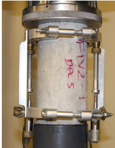
Figure 3-6: Cylinder compression test
