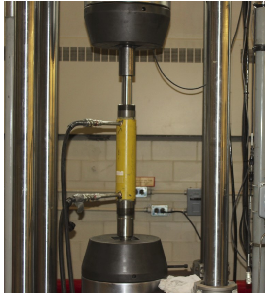
Figure 3-18: Friction test for the hydraulic jacks
