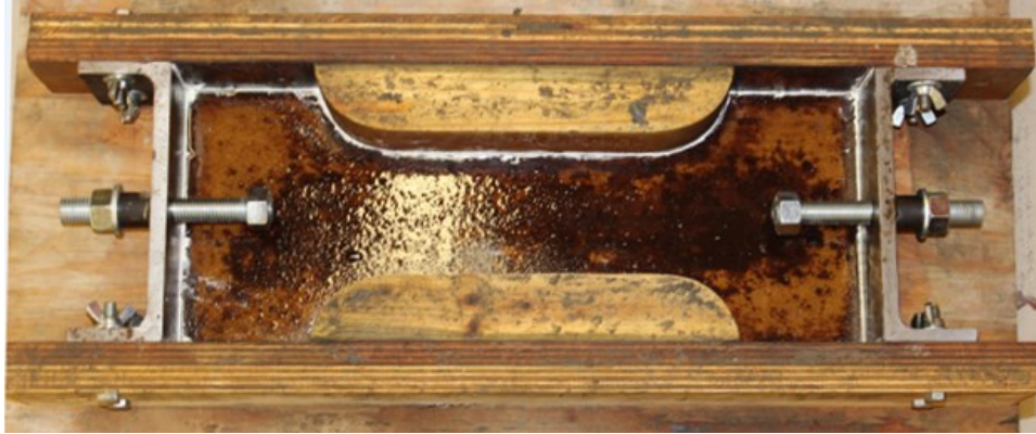
Figure 3-9: Dogbone forms with \frac{3}{4} " threaded rods locked in
