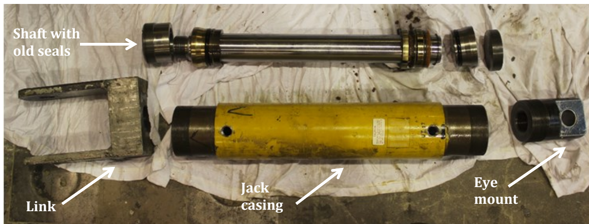
Figure 3-16: Disassembled hydraulic jack
