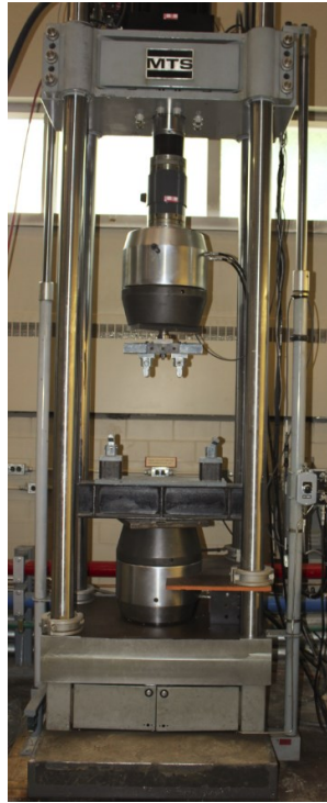
Figure 3-14: MTS Four Post Test Machine
