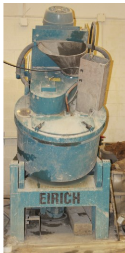
Figure 3-2: Eirich Concrete Mixer (150 litre capacity)
